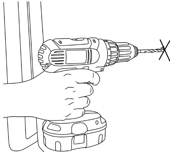
Reposition stand and secure unit to wall using the four lag screws (M) and washers (G) supplied and a 1/2" (or 13mm) driver to tighten. For masonry, install lag shields (O) prior to bolting in position.
