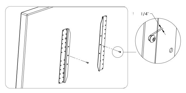
Two people are needed to install the display on the stand. Position alignment screw into the "key hole" slot as shown and continue holding display.
