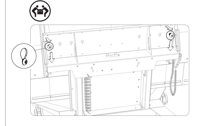
Immediately use (4) "H" screws to affix the mounting brackets to the cart-side mechanism as shown. Tighten all screws firmly.
