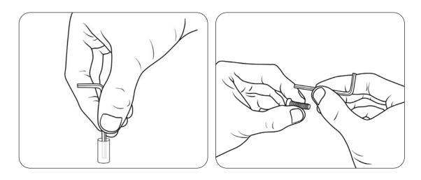
Install interface mounting brackets (O) onto display as shown using supplied phillips screws (A-G) or screws specified by the display manufacturer. **Hand tighten first to confirm thread and depth match.** Note: Affix display brackets "Ears-Out" as shown
