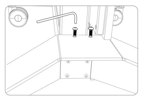
There are 6 "I" screws per leg. The fifth screw is installed on the top of the leg as shown above.
