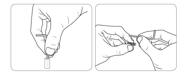
Install interface mounting brackets (J) onto display as shown using supplied phillips screws (A or B) or screws specified by the display manufacturer. **Hand tighten first to confirm thread and depth match.** Note: Affix display brackets "Ears-Out" as shown
